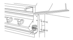
2) Push the BBQ back into its position in the bench, and attach rear cover by lifting the hood slightly, and placing the trim strip in between the body and the hood:
