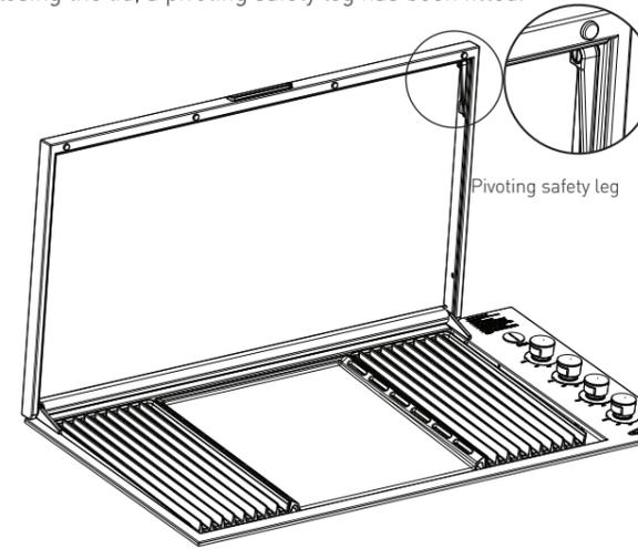
When closing the lid the safety leg will pivot forward and rest against the trim surface to prevent the lid closing. After ensuring the gas has been turned off, to fully close the lid, the leg needs to be rotated backwards.
