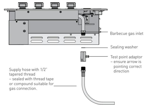
After connecting the barbecue to an Universal LPG gas supply, test the operation of the appliance:
