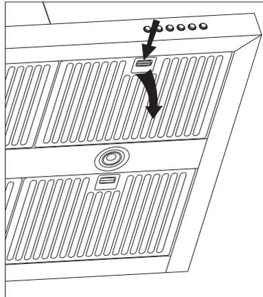
Unscrew all the 4 screws on lateral sides, then open the inner filter for cleaning.
