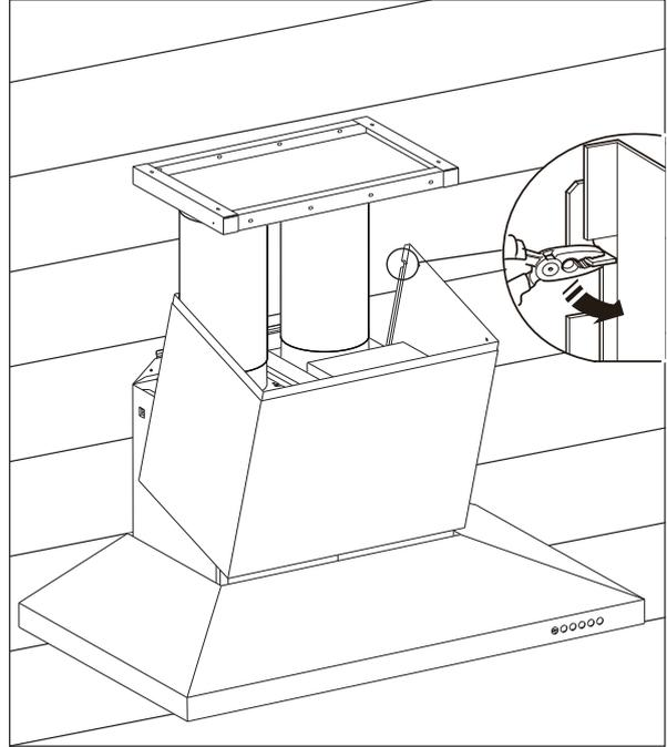
10. Slide telescopic flue cover to upper position and fix with screws provided.
