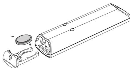
Insert the battery (battery type: Cr2032), then fix the battery bracket with the screw.
