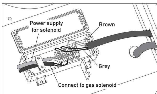
**Circuit connection for gas solenoid valve:**
