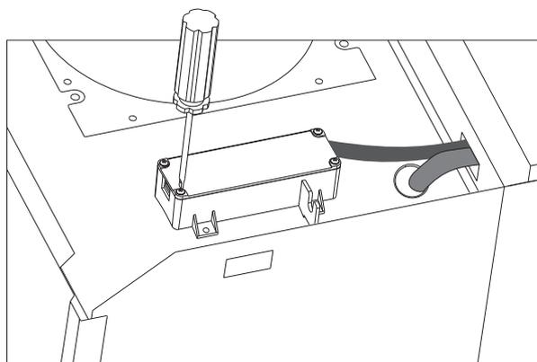
7. Connect the wire as following picture show, then close the box cover and fix it with screws.
