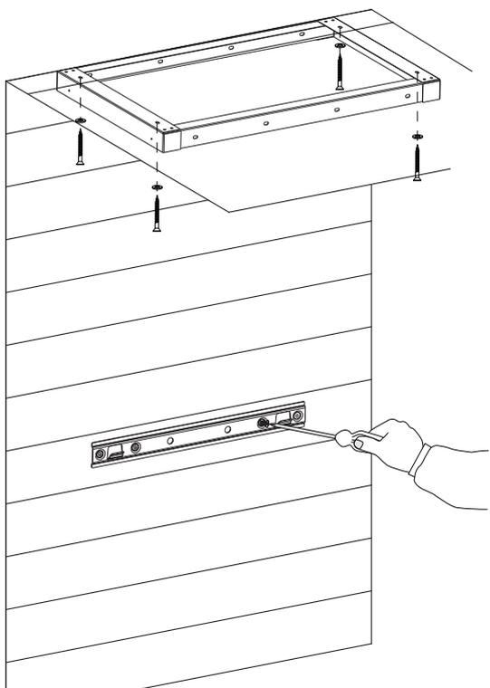
4. Remove protective plastic film, if present, from the hood body and hang on the wall bracket. Install the two anti-tilt fasteners.
