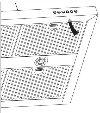
2. Pull down the filter lock level and then pull the filter assembly down and out of the hood.
